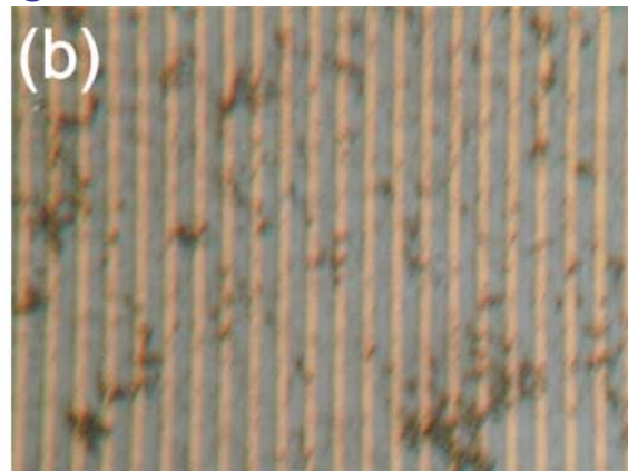
SEM image of the bridge formed by enlarged gold particles.
